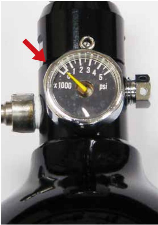
**POSSIBLE CAUSE:** insufficient air supply ( HPA)
