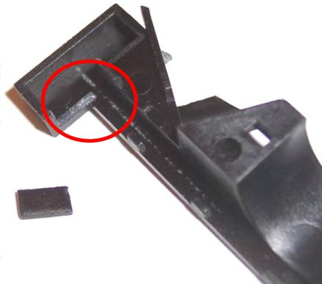
Step Two – Using a razor knife, relieve this tab on the inside of the right grip clamshell to allow the trigger sensor to fit inside.
