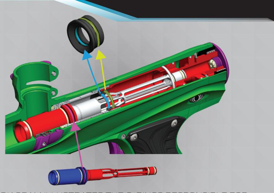
THIS DIAGRAM ILLUSTRATES THE O-RINGS RESPONSIBLE FOR AIR LEAKING FROM INSIDE THE FACE OF THE BOLT.
