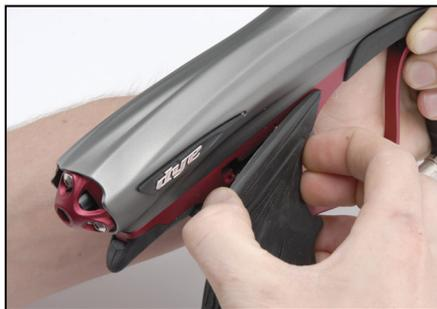
1. Pull the upper back corner of the grips away from the gripframe with your thumb. Allowing the rear tabs to clear the frame.
