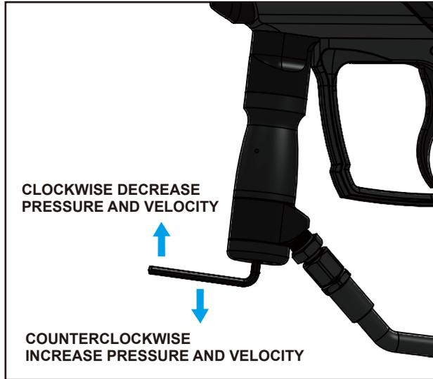
Adjusting the regulator will change the amount of pressure entering the marker. Regulators are preset for optimum performance from the factory and most adjustments should be made through the rear velocity adjuster.
