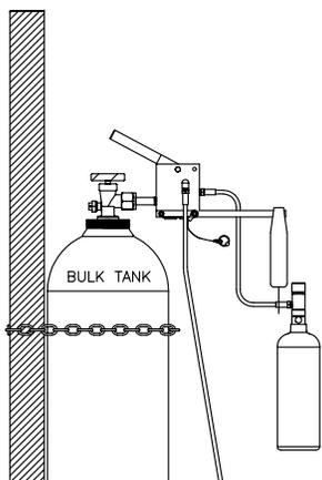
10. Unhook the bottle & hose from the scale and turn the Depressor Knob counterclockwise at least 2 full turns. This should allow the bottle's pin valve to be fully closed.
