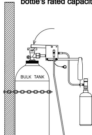
9. Allow the control lever to return to it's neutral position.
