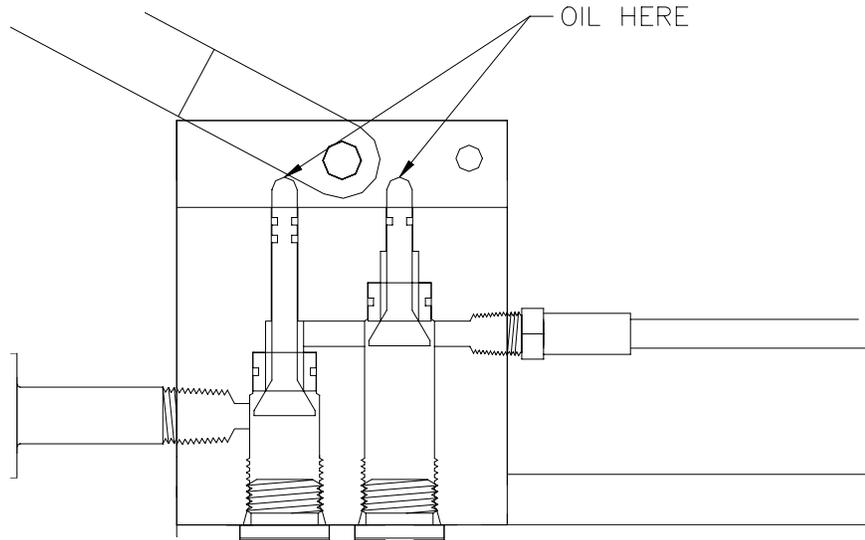
The other item that wants occasional lubing is the "O" ring in the Universal Fill Adapter. On at least a daily basis, apply a couple of drops of oil to the depressor pin in the UFA, in order to keep this "O" ring lubricated.
