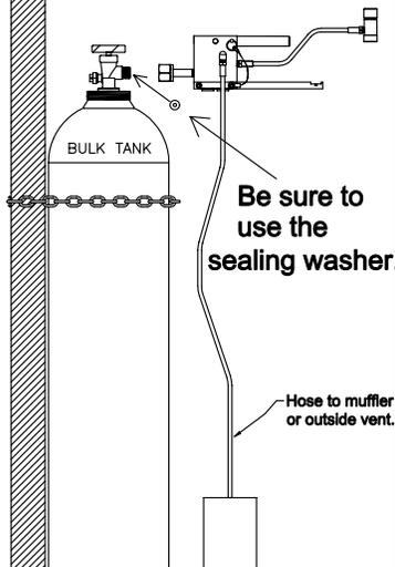
3. Make sure the control lever is still locked in the "Dump" position.....
