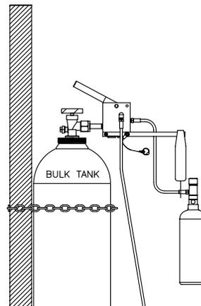
8. Move the control lever to the FILL position and watch the scale.
