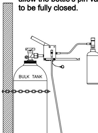
11. Move the control lever to the DUMP position to drain any residual CO2 from the hose.
