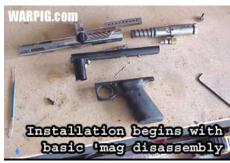
For someone who is familiar with properly maintaining their Automag, armed with the knowledge from Airgun Design's maintenance video, installing the Hyperframe is not a terribly challenging task. It starts with disassembly of the
