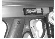
Remove the 2 screws that hold the battery cover in place. Connect the battery to the terminal and place the battery inside the frame (or tray) carefully being sure that the black and red wires to the terminal are forward and are toward the bottom. Make sure that there are no abrupt kinks and the wires are comfortably placed, do not force them into place. Replace the cover and 2 screws.
