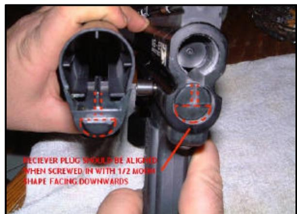
at the rear of the A1/A2 models which do not have a velocity screw. You can adjust the velocity by turning the complete striker plug assembly or by adjusting the length of your spring on this
