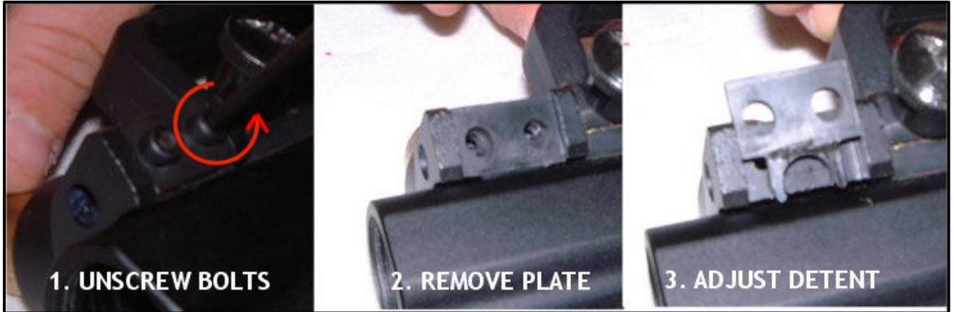
Unscrew the retaining bolts holding the ball detent plate, then remove the plate so that you have easy access to the rubber detent – depending on the size of paintball being used, and/or operational problem being experienced you will need to judge whether to adjust the ball detent for more or less resistance on the ball.
