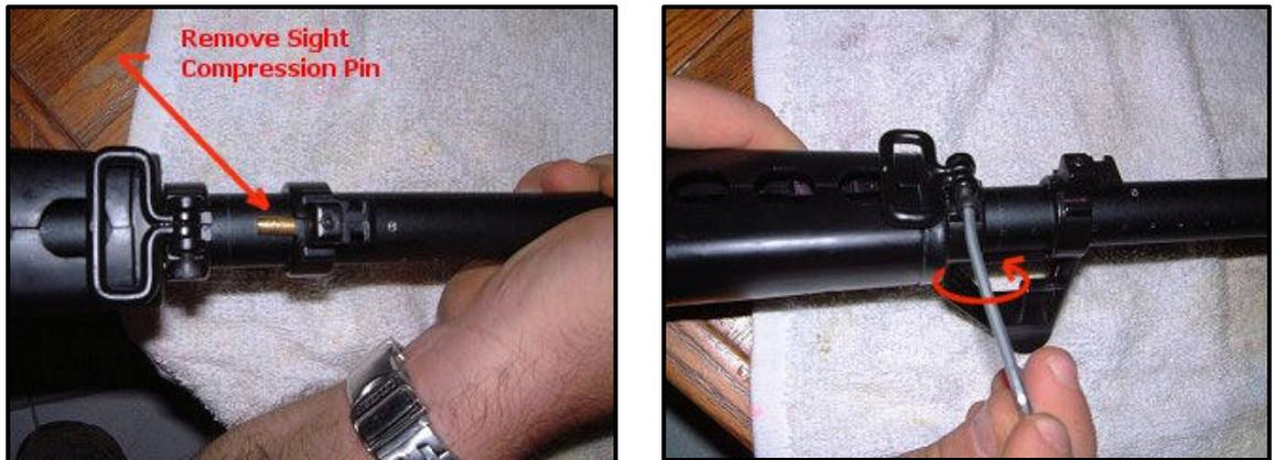
Loosen the lug that holds the sight compression pin, then loosen the the bolt that holds the sling attachment ring Next loosen the lugs on the rear section of the hand guards – the whole assembly should be loose enough to rotate and adjust so its properly aligned for sighting – make sure the barrel is tightly set into the receiver before doing the alignment – then retighten all screws
