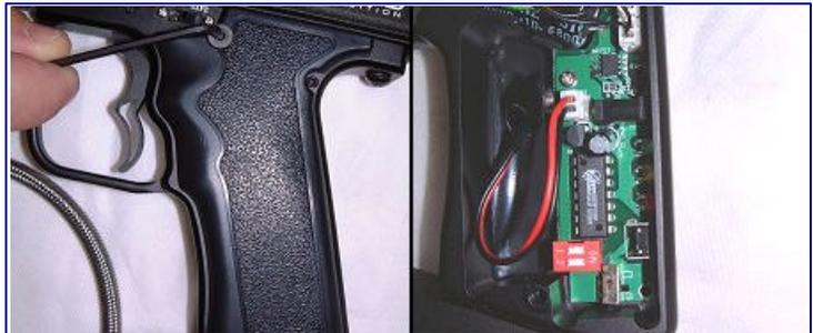
3. Use a rechargeable 9.6v battery to power the trigger frame. Insert the battery into the frame, and ensure that no wires are loose, pinched or unsecured before replacing the frame cover.
