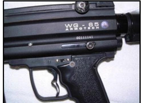
10. Turn the safety switch to the FIRE position and then squeeze the trigger with an even pressure. The cocking knob should snap forward into the un-cocked position. You have just dry-fired your Armotech marker. Do this a few times until you are comfortable with this operation and the feel of the marker when cocking, and firing it.
