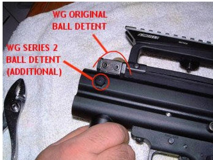
In some cases it, may be required to remove the original ball detent system to avoid ball breakage problems –
