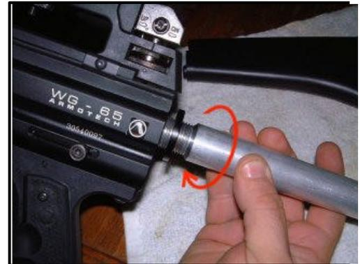
Stock removal on the A1/A2 model of the WG65
