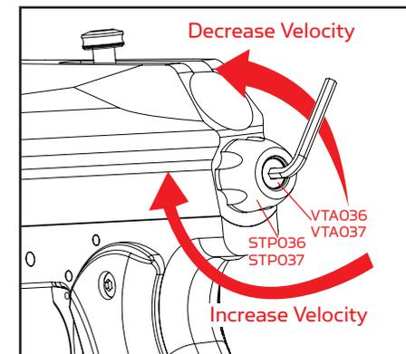
To **INCREASE** your velocity FPS (Feet Per Second) using the Allen wrench turn the Velocity Adjuster / Spring Guide clockwise.
