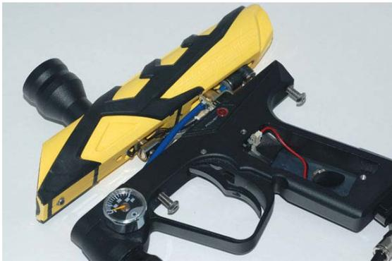
5. Remove the front pneumatic fitting with a 1/8" Allen wrench. Make sure to remove the pneumatic fitting from the hose afterwards and set it aside.
