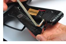
Unscrew regulator from frame (degass marker first)
