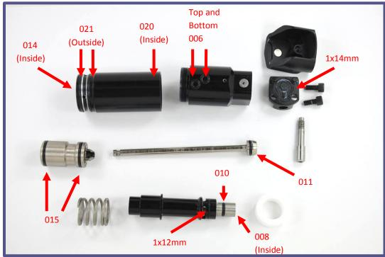
SUPERCHARGED ENGINE O-RING LOCATIONS
