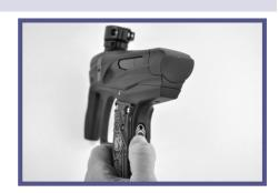
To power off marker: Press and hold the power button for 1.5 seconds, until the LED turns off, then release. Every time the marker is turned on, the eyes are enabled. The marker can be turned off regardless of the state of the eyes.
