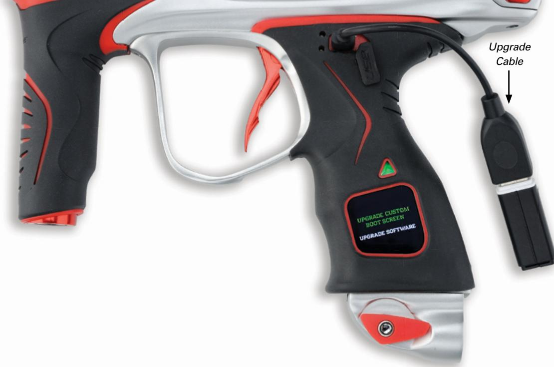
You can customize the boot screen on your M2 with any photo you like. The full color provides remarkable detail and image resolution. Before you can download a photo onto the board it will first need to be converted to a .bmp file sized 128 x 128 pixels. You can use any number of free online programs such as the one listed below to convert your photo. <http://image.online-convert.com/convert-to-bmp>
