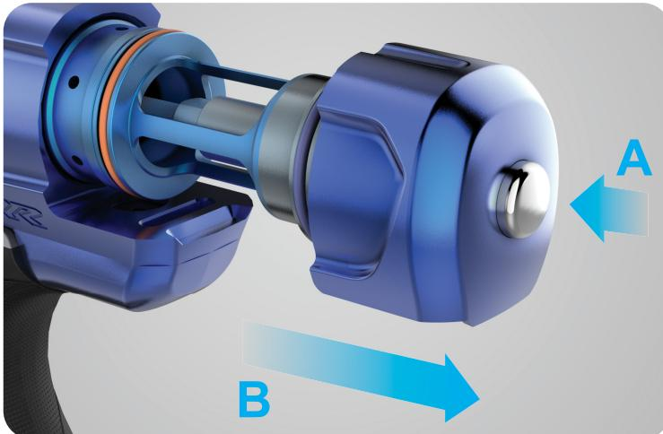
To remove the ARC+ Bolt, secure the back cap between index and middle finger and depress the push button. With the push button fully-depressed, pull firmly back to remove the ARC+ Bolt.
