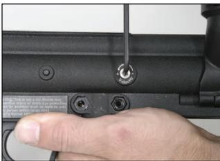
Figure 6.  $\frac{1}{8}$ " allen wrench is used to adjust velocity.
