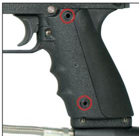
Unscrew the 2 clip bolts with a 5/32 allen key, or remove the 2 fieldstrip clip pins to release AEC frame.
