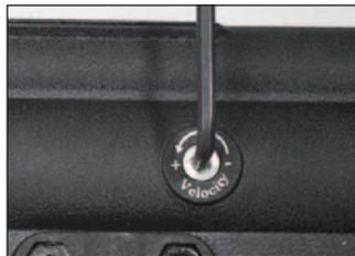
Figure 7. Clockwise decreases velocity. Counterclockwise increases velocity.
