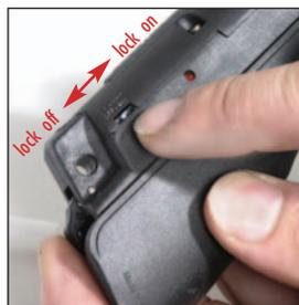
Turn on Tournament Lock by pushing the button up and turn it off by pushing the button down.
