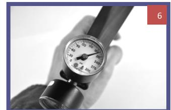
NOTE: The supercharged engine which has a red blast guide will run at slightly lower pressures. Starting at 75 PSI on the LPR to get reliable cycling is recommended at a minimum. While the HPR setting helps establish initial operations always use a chronograph to ensure you are firing within limits that are legal and safe for your playing area.
