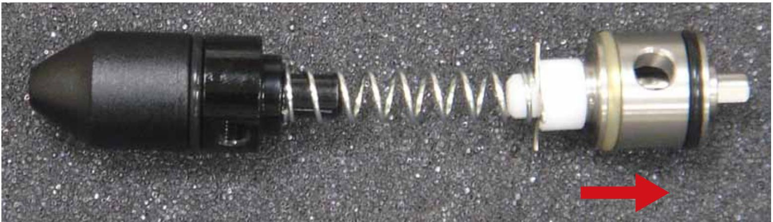
**POSSIBLE CAUSE:** Cup Seal Guide is jammed in the valve
