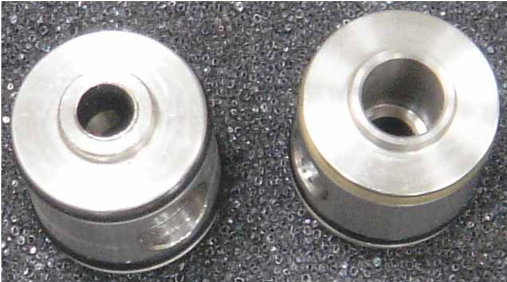
**POSSIBLE CAUSE:** Valve installed incorrectly
