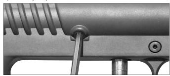
To adjust the velocity use the small allen wrench included with your gun. The velocity adjustment screw is located on left side receiver at a 45° angle. To adjust the velocity down, turn the screw inward or clockwise. To turn the velocity up, turn the screw out or counterclockwise.
