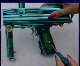
reading starts to drop turn the pot back anti-clockwise a few degrees and ensure your chrono reading is consistent, the Angel is now at its most efficient setting. If you turn the valve dwell down too much you will starve the valve of gas to propel the ball at the specified velocity. If the Dwell is set too high the gun will sound very loud and inefficient.
