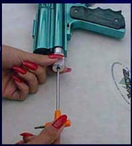
signature change as the snap ring tightens and eventually the gun will stop firing and you will hear a 'clicking' noise. When you hear this 'clicking' turn the snap ring 1/3 to 1/2 turn anti-clockwise. Your ram snap ring is now in the correct position and your problem will have been deleted. It is far easier to complete this task with a Ram Adjuster Tool.
