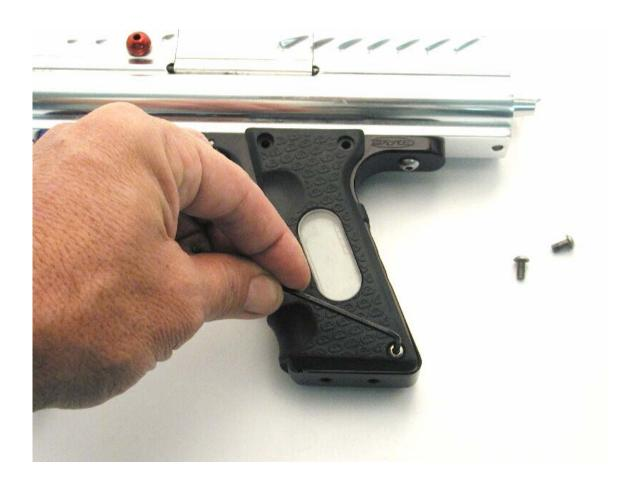
Remove the three screws from the LCD side of the grip.
