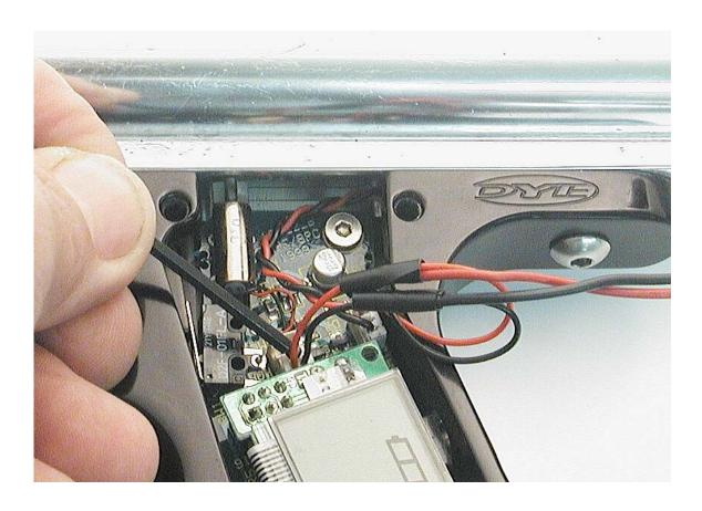
Reconnect the plug. Note that the plug only goes in one way! (The red wire on left in this view.)
