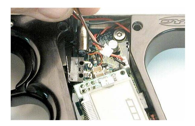
Remove the plug, but don't pull it out by the wires!
