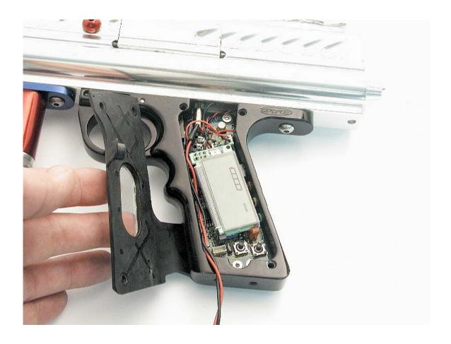
Run the harness down and towards the front of the grip as shown. Close up the grip while aligning the wire with the notch you made.
