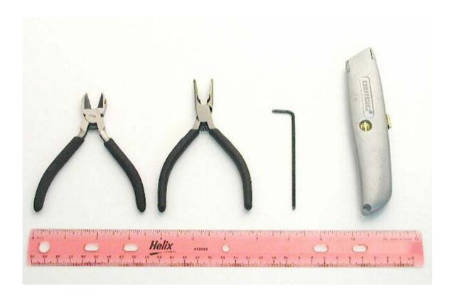
Wire strippers, Needle-nose pliers, 3/32 allen wrench, utility knife, 12 inch ruler.
