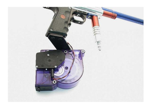
Make sure your Warp is jumpered for positive input; the jumper in the three position header should be in the middle position. Plug it in, turn on the marker and it should spin every time you pull the trigger!
