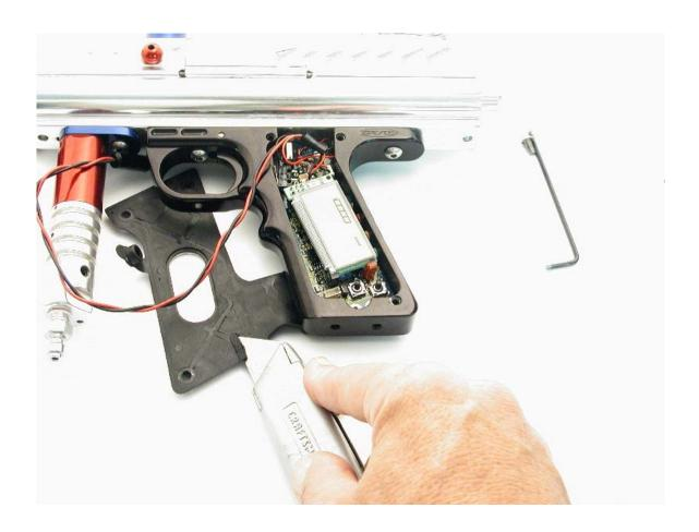
With the utility knife, carefully make a small "V" shaped notch ½ inch long on the inside of the grip as shown. Be careful not to cut all the way through!
