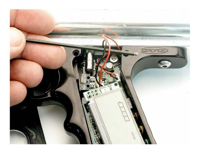
Here are the two wires that we will tap into. We will accomplish this by just skinning the insulation back and not cutting the wires themselves.
