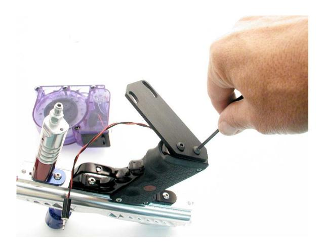
We are setting this marker up for a right handed player and hanging our Warp off the left hand side of the marker. Note the un-slotted side of the Warp Mounting Bracket connects to the grip frame. You would normally bolt on your air system here too, but we have omitted it for clarity.
