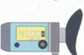
This display shows that the battery is low on power and needs replacing. The batteries have only 10% of their power left when the battery icon appears. If no display is possible you must replace the batteries as they are totally discharged of power.
