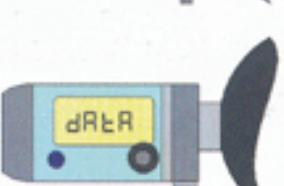
This display may appear for 1 second when the menu is being scrolled through, this indicates that new data is being calculated and checked prior to displaying the data.
