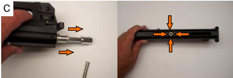
C— Tilt the upper body to slide the bolt (part # 15) towards the back of the marker and remove by pulling towards the direction shown.
