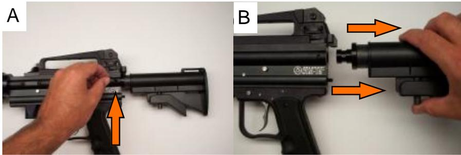
A—Loosen stock retaining screw (part #19) With a 3mm Allen Key
