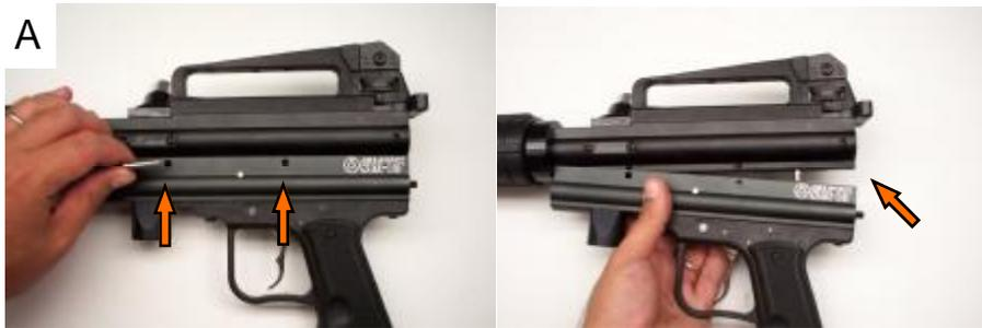
A—Squeeze gun body together and pull out the body pins (part #14)
