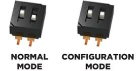
**NOTE:** You cannot turn your marker off with the power button when the marker is in configuration mode. You must first set DIP switch 2 to the OFF position.
