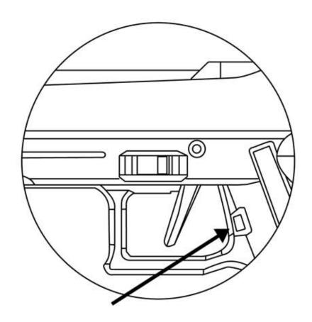
When there is CO2 in the canister, the magazine will eject from the handle. When there is no CO2, you must pull the magazine free.
