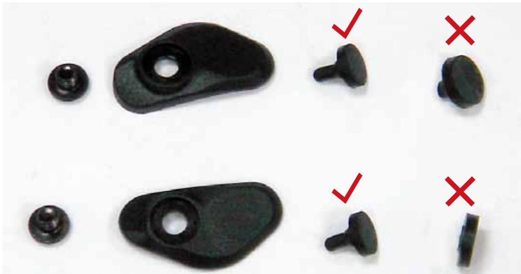
**POSSIBLE CAUSE: Ball Detents are damaged**
