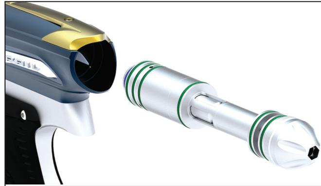
inside the supply chamber causes the bolt to start moving forward. Once the bolt has moved about half way forward, the tail of the bolt closes the input into the supply chamber. Once the Bolt reaches the forward point, the valve of the REFLEX RAIL™ Bolt is opened and air inside the supply chamber goes through the Bolt and fires the paintball.
