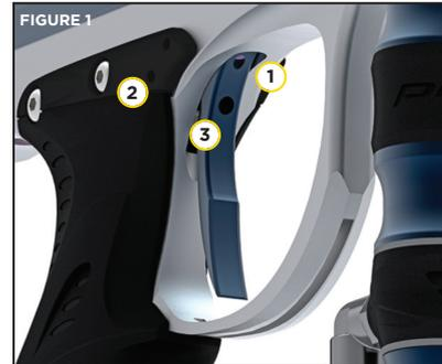
The Trigger's forward travel and over travel are fully adjustable so that the user can fine-tune the trigger to his/her exact preference. To adjust the trigger you will need an .050" and 5/64" Allen key. There is one adjustment screw located on the right side of the Ultralite frame behind the sticky grip, one adjustment screw located in the top of the trigger, and one adjustment screw behind the trigger.
