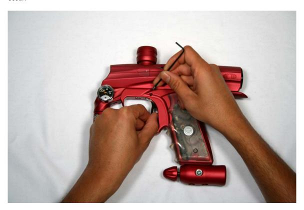
**STEP 8**Using a .050 hex Allen wrench adjust trigger spring, switch contact, and rear travel screws.
