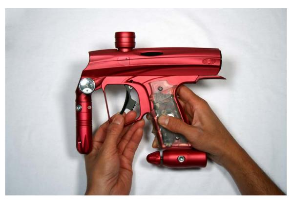
**STEP 3**Using the .050 hex Allen wrench remove stock trigger spring assembly.
