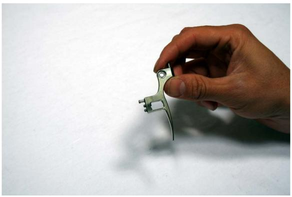
**STEP 5**Install trigger spacer (provided with trigger) with stepped side facing bearing into trigger.
