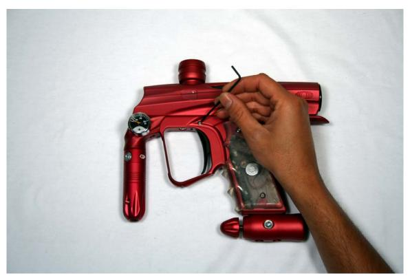
**STEP 2**Remove stock trigger through grip frame.
