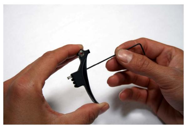
**STEP 4**Install spring assembly into new CP trigger.
