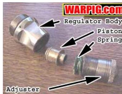
Since the relief valve vents excess pressure between the regulator and the paintgun, the output pressure gauge can further diagnose air venting from the relief valve. If the pressure is normal, it would indicate a damaged relief valve. Unusually high output pressure indicates a dirty or damaged regulator pin.
