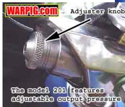
the tank gauge, low pressure output, low pressure gauge, and fill nipple. At the end of the regulator is the adjuster. It's knurled edges make hand adjustment possible, but tuning is most easily done with a 3/16" allen wrench.
