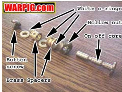
With the valve core removed, a 3/16" allen wrench can be used to remove the hollow nut which holds all of the on/off seals in place. An o-ring pick can be used to remove each of the three white o-rings and two brass spacers which seal the valve. A fourth o-
