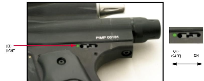
**A BLINKING OR SOLID LIGHT INDICATES THE MARKER IS LIVE. IF THE SWITCH IS TURNED TO THE ON POSITION AND THE LED DOES NOT LIGHT UP OR CONTINUALLY STROBES, THE BATTERY MAY NEED TO BE REPLACED.**
