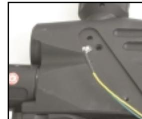
The eyes can be gently removed and cleaned by factory trained technicians only. Broken or pinched wires are not covered under the warranty.
