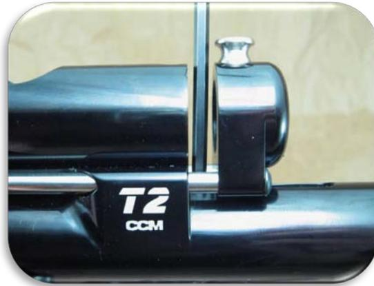
Turn the Allen key clockwise to *lower* the lug (allow the marker to fire with a longer trigger pull – or during auto trigger – later in the cycle) and to the anticlockwise to *raise* the lug (allow the marker to fire with a shorter trigger pull - or during auto trigger - earlier in the cycle).
