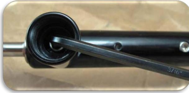
8. The VRA has one static o-ring – which I lightly lubricate (Dow 55) upon reassembly.
