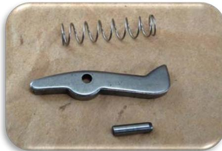
9. Inspect the Sear to see if it has wear where the lug catches. (Notice the slight wear on this sear.) Wear can cause the marker to 'skip' (not recock from time to time) or be VERY hard to time the auto trigger. Replace this if wear is evident or malfunctions are occurring. This should not need to be done often and perhaps will never need to be replaced on your marker.
