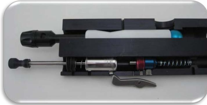
*Note: This is a cutaway of a CCM Series 5, a full block marker. The T2 works nearly the same way and seeing a cut away will help you understand what is happening inside your marker. The T2 is nearly identical to the Series 5 and 6 markers with the exception of being 'half blocked'. This is the marker cocked with a ball in the chamber.*
