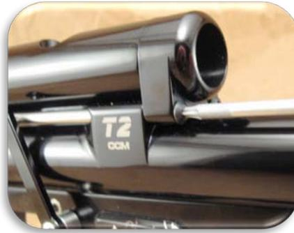
**Note:** Be very careful when replacing these screws. Use blue loc-tite and do not over tighten. Finger tight allows for smooth movement of the backblock and bolt. Over tightening of the back block screws can cause binding *once* the bolt is installed.
