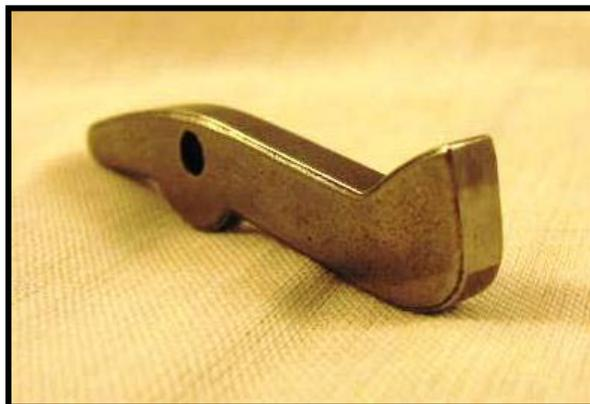
10. Remove the Trigger Shoulder Bolt and slide the trigger from the frame (shown with the top Allen key). Be sure not to over tighten the Trigger Shoulder Bolt. Over tightening can cause drag on the trigger.
