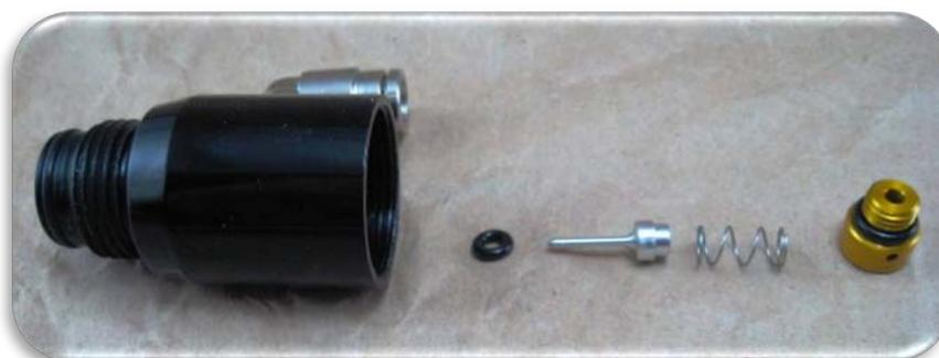
4. Clean (use your Q-tips® in all the appropriate places on the regulator top) and replace the regulator Pin O-Ring if necessary. Apply a light coat of oil to these parts and replace them.
