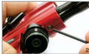
Remove LPR Retaining Screw
