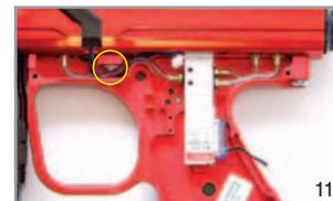
Loosen Front Frame Retaining Screw
