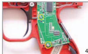
Remove Board Retaining Screws
