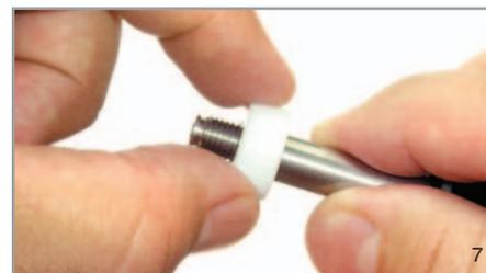
Remove Delrin Bolt Pin Receiver Spacer
