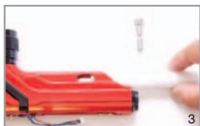
Lift Bolt Pin and Remove Bolt
