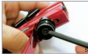
Remove ASA Retaining Screw
