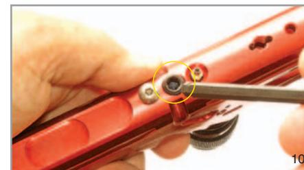
Remove Valve Retaining Screw
