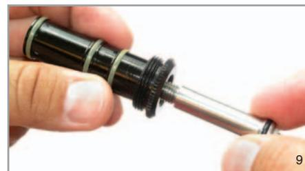
Tilt Ram Sleeve Up and Remove Ram from Rear
