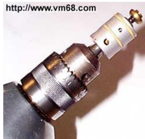
Make sure to leave a little space between the valve and cup seal.
