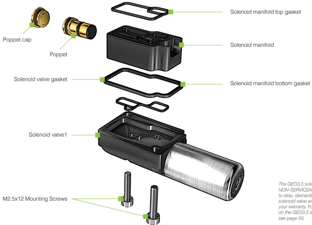
*The GEO3.5 solenoid valve is NON-SERVICEABLE. Any attempt to strip, dismantle or service the solenoid valve will immediately void your warranty. For more information on the GEO3.5 solenoid valve please see page 56.*
