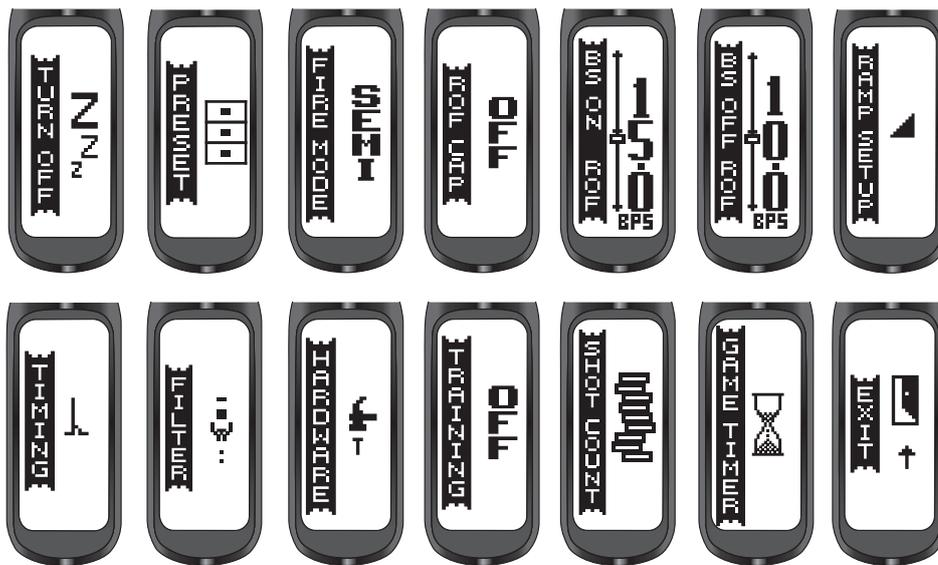
The Main menu contains both editable parameters and sub-menus which contain editable parameters. Some of these parameters affect the way the GEO3.5 shoots and are tournament locked as standard from the factory.<sup>1</sup>
