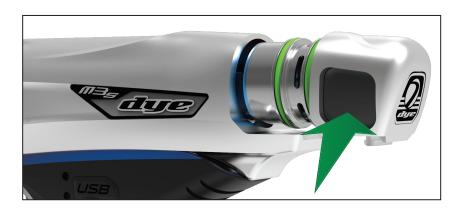
To remove the bolt, grab the bolt back cap with your right hand. Push the bolt release button, located on the left side of the bolt back cap, with your thumb. With the bolt release button depressed pull firmly back on the bolt.
