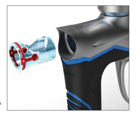
remove the eye pipe/detent system from the front of the M3s and unclip the detents for a thorough cleaning. Reinstall the detents, and eye pipe after you have sufficiently cleaned the detents and breech.
