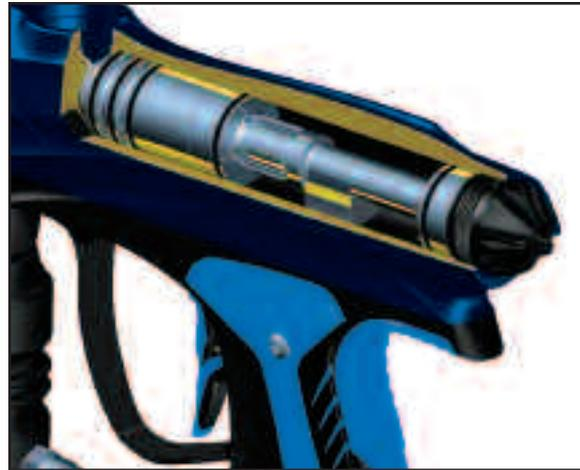
The RAIL™ BOLT is the main component of the PMR marker. In order to achieve the best possible performance of the PMR it is essential that the RAIL™ BOLT is kept clean, well lubed and in good working order.
