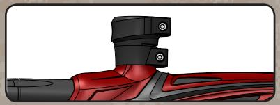
03 LOADER/PAINT: Insert a paintball loader (not included) into the eNMEy<sup>™</sup> feedneck. High-performance electronic loaders allow for higher rates of fire and minimal paint breakage. Align the loader and tighten both its top and bottom clamps with a 7/64-inch allen wrench. Do not fill the loader with paint until ready to fire at a paintball field. Use of high-quality, fresh paintballs will result in best performance.
