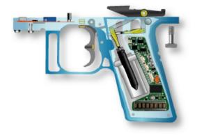
The Grip Frame contains all of the electronics that run the X-mag.
