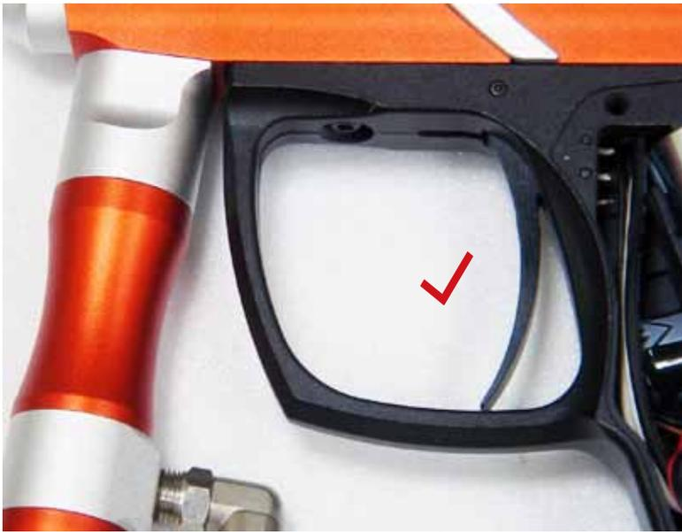
Back out the trigger leave some space between the trigger and micro switch.
