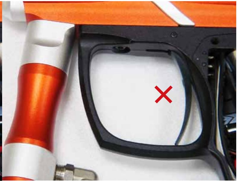
Too far back and too close to the micro switch at the back of the trigger.
