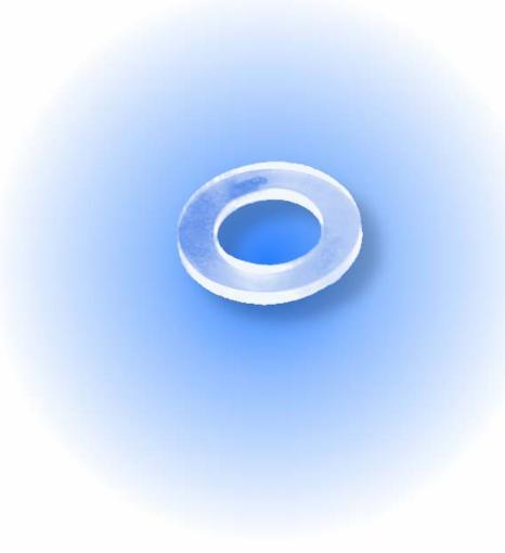
This clear urethane washer sits at the base of your power tube. When the bolt returns, it hits this to decelerate. This bumper is a little softer than the standard blue bumper for the higher firing rate of the Retro Valve. The bumper should be replaced about once a year. One Included in the Parts Kit.
