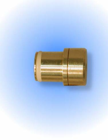
The Regulator Piston comes as an assembly that has a built-in blow off valve. Do not disassemble! Replace this part when air is venting out the back of the marker and you are shooting less than 300 FPS.
